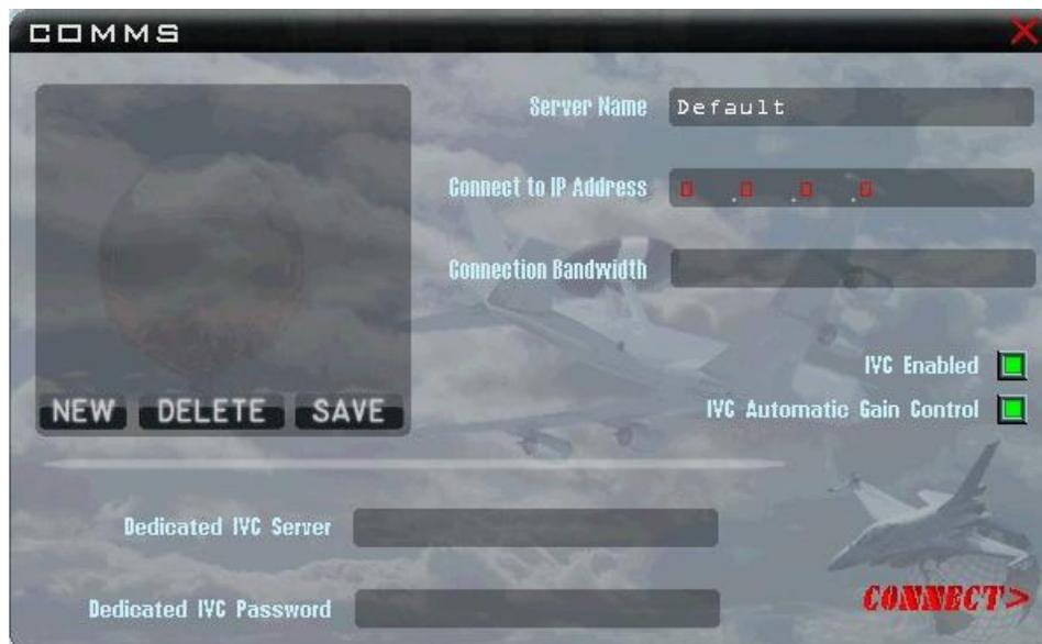
FBMS mimics AF's ease of online multiplayer connections but is based upon a proven third party multiplayer system known as RakNet. Once in the sim go to the "comms" menu option along the top and in the window you enter the Server Name (optional), IP of the host (Connect to IP Address) and the appropriate bandwidth (Connection Bandwidth). The connection bandwidth will usually be decided by the host depending upon his connection speed.
